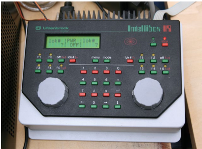
A model railway controller, such as the Intellibox in the picture, allows for controlling a model railway both locally and with a computer.
